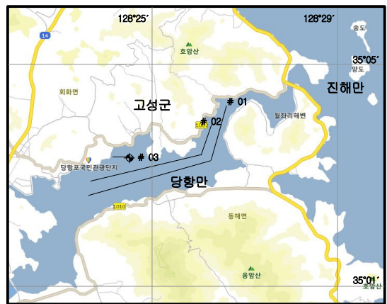
Figure 2: Survey lines of chirp sub-bottom profiling (2-16 kHz) and the coring position (◆).
