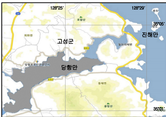
Figure 6: Distribution map of gas-bearing sediments (diagonal lines) expected by SBP survey.
