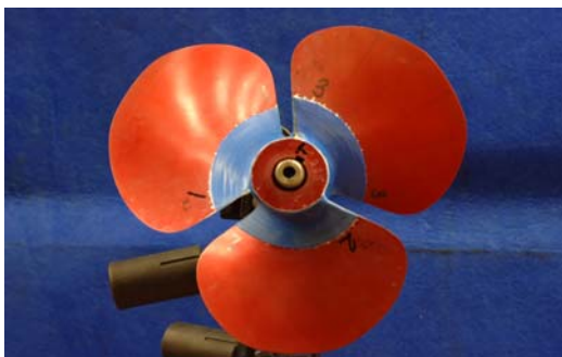
Fig. 7 Preparation of model propeller coated with paint A
