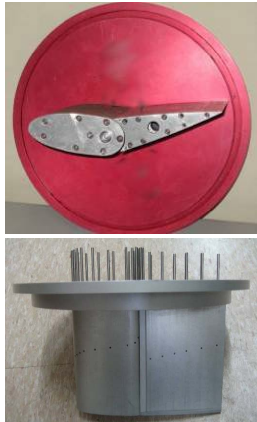
Fig. 4 Pintle section model for cavitation visualization(upper) and surface pressure measurement(lower)
