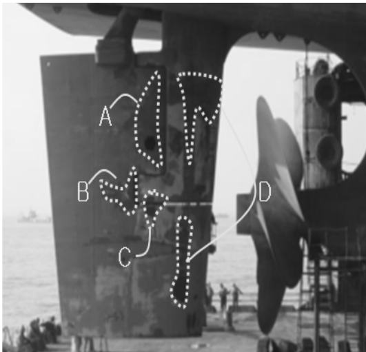
Fig. 1 The erosion by cavitation on horn-type rudder(Seo et al. 2009b)
