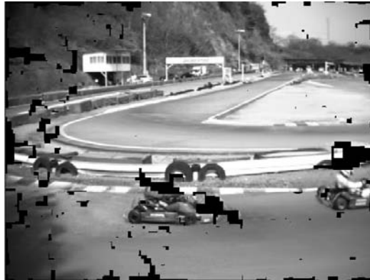
Fig. 11. SI frame after MCTI step, which has multiple holes
