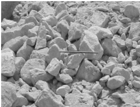
Fig. 12. This figure reveals good and uniform fragmentation along the back rows of the blasts fired on skewed V-type firing pattern. Fragmentation along the back rows is very consequential in governing the success of any blasting program. Linear scale 0.5 m long appears in the picture.
