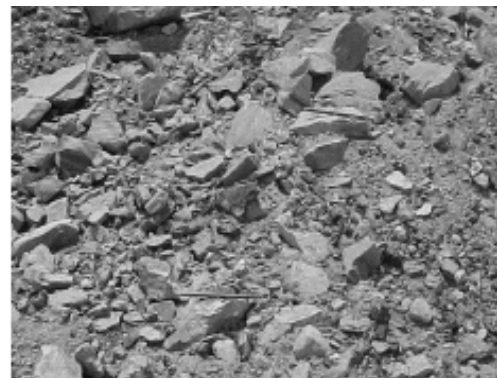
Fig. 10. This figure demonstrates that the muck-piles fired on skewed V-type firing pattern, yielded finer fragmentation with better uniformity of fragment sizes within the muck pile in comparison to the blasts fired on straight-V type firing patterns. The linear scales, as appearing in the image frame, were 0.5 m long.
