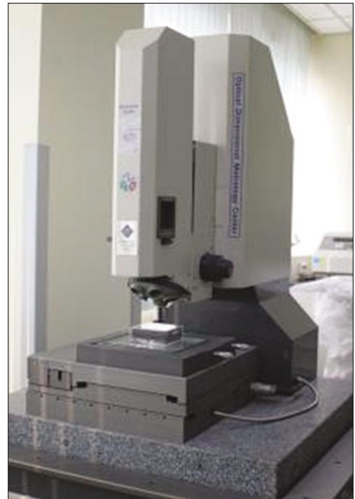
Fig. 1. Accura 2000®, a non-contact, non-destructive, optical 3-dimensional surface analysis system.
