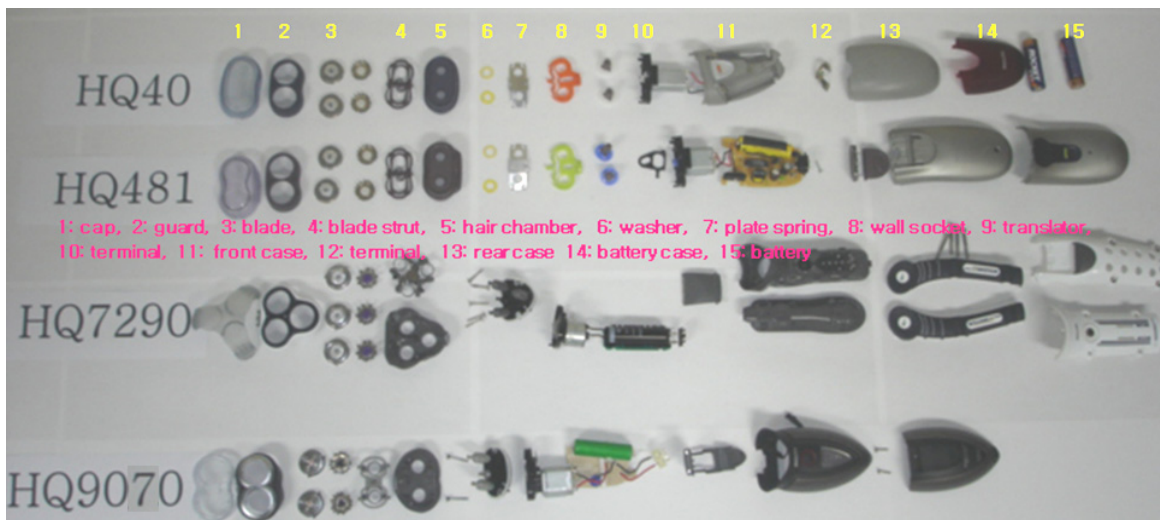
Note) Part name: 1: cap, 2: guard, 3: blade, 4: blade strut, 5: hair chamber, 6: washer, 7: plate spring, 8: wall socket, 9: translator, 10: terminal, 11: front case, 12: terminal, 13: rear case, 14: battery case, 15: battery.
