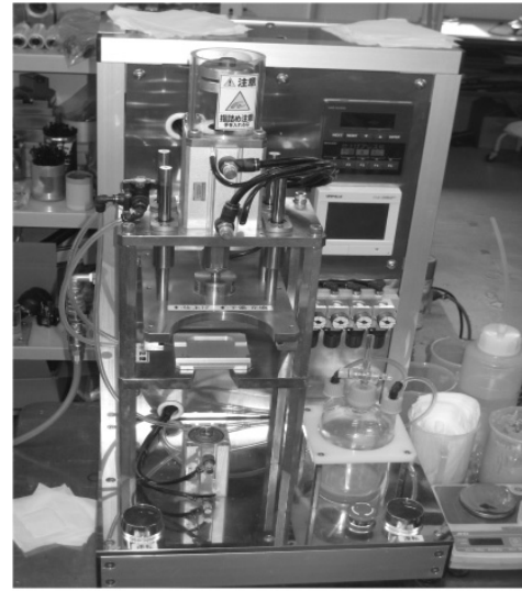
Figure 1. Wet slurry press machine.
