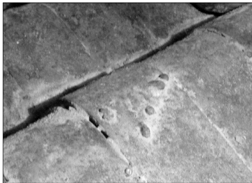
[Fig. 4] Damage to the grate and the refractories of incineration facilities.
