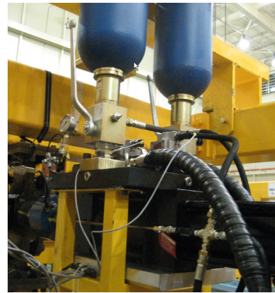
Fig.3 Hydraulic actuator for centrifugal load realization
