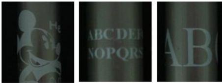
Fig. 9 Various marking results on cylindrical parts
