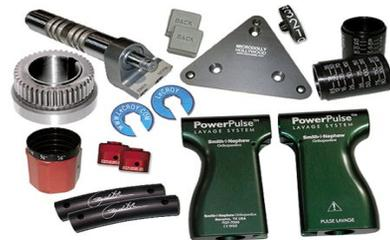
Fig. 1 Laser marking examples
