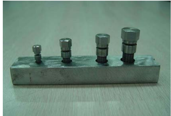
Fig. 2 Various diameters of reverse screw
