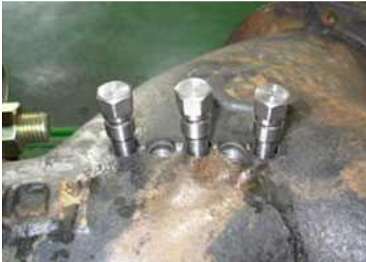
Fig. 1 Casting crack repairing using reverse screws
