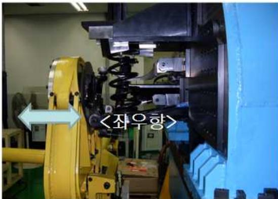
**Fig. 4 Test operation condition of a 1/4 car**
