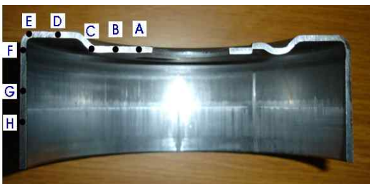
Fig. 10 Section view of Drum Clutch Hub and location of dimension measurement
