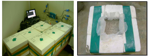
Figure 10. Adiabatic temperature rise test Chamber (300×300×300mm)
