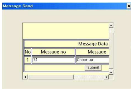
Fig. 8. An MFC dialog containing the web browser control for message downloads. The dialog-based application navigated this page, and displayed the therapist’s message to the patient.
