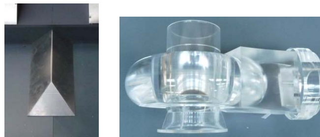
Fig. 6 Modeled 90°-floor-splitter and submersible motor pump
