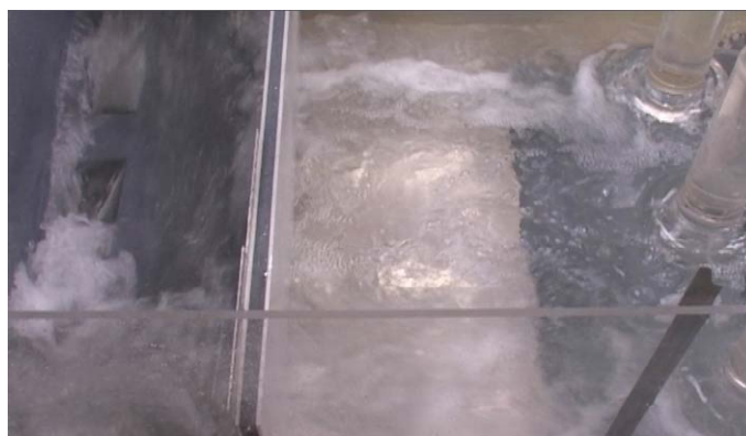
Fig. 12 High air entrainment and foam formation (phase 1)
