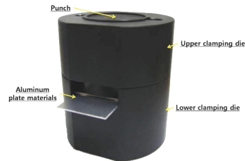
Fig. 4 Assembly die of extru-rileting welding process
