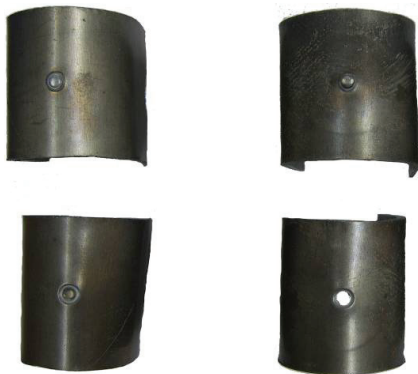
(a) Type one (b) Type two Fig.12 Kinds of tensile fracture (T=520 °C)
