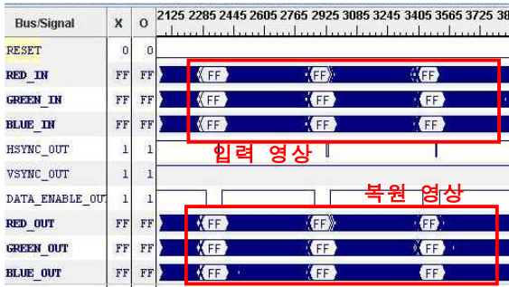
Fig. 10. The result of video data waveform by ChipScope
