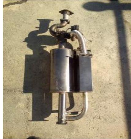
Figure 2: Photograph of smoke reduction system of the exhaust gas suction type
