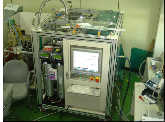
Fig. 4 Leak test equipment
