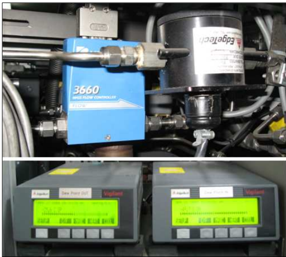
Fig. 9 Dewpoint measurement setup
