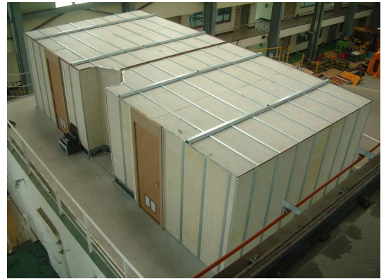
Fig. 3 Unit cabin installed in the deckhouse mock-up
