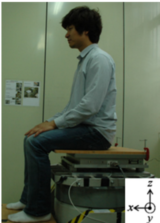
Fig. 2 Photographic representation of exciter and subject sitting on the rigid seat
