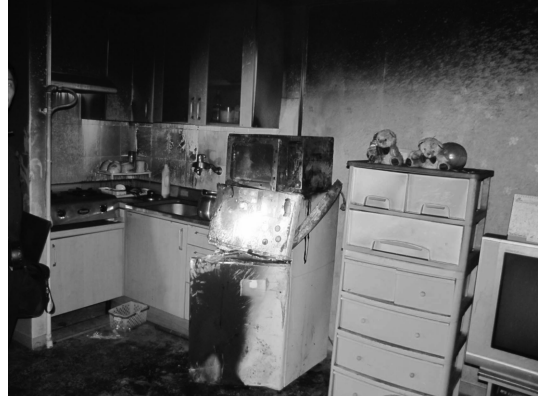
Figure 3. Burned feature of refrigerator' outside.
