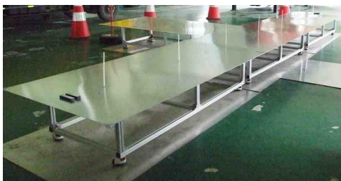
그림 6 축소 모의실험을 위한 축소 모의선로(50:1) Fig. 6 Photograph of the transmission line for which the reduced simulation test was performed (50:1)
