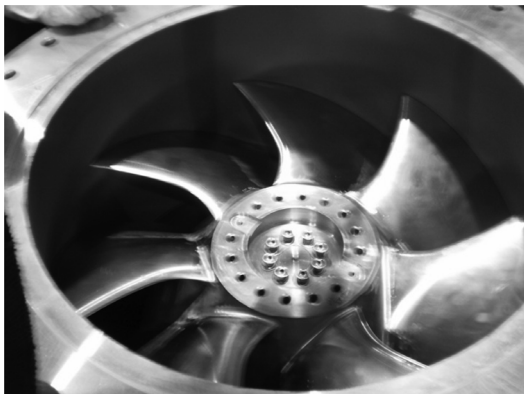
Fig. 2 Assembling of impeller and impeller housing
