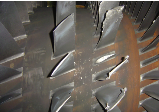
Fig. 4 Damaged compressor blades
