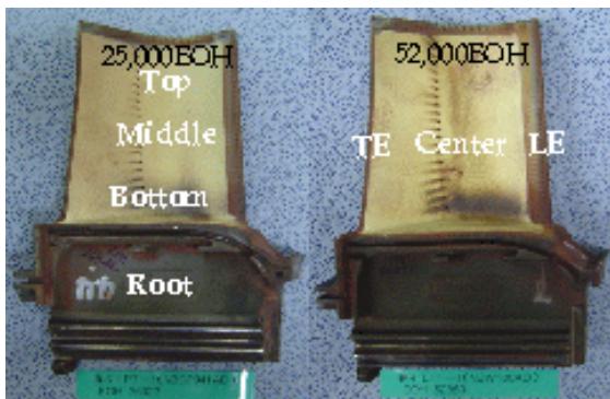
Fig. 1 Macroscopic view of the used blades
