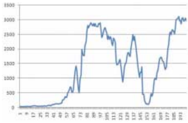
Fig. 3. Line analysis result of EPMA (Electron Probe Micro Analyzer) data of Ca at 6 week.
