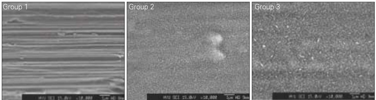
Fig. 4. FESEM (Field Emission Scanning Electron Microscope) findings of implant surface. Group 1: Machined, Group 2: Treated with alkali and heat in atmosphere, Group 3: Treated with alkali and heat in vacuum.
