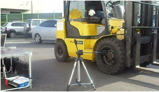
Fig. 7 View of squeal measurement test using a forklift
