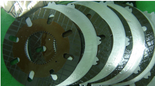
Fig. 3 Brake components consisting with pairs of plate-friction and plate
