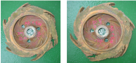
Fig. 7 Wear and tear on the impeller's shape by cavitation
