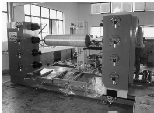
Fig. 2. Photograph of the horizontal type filament winding machine.
