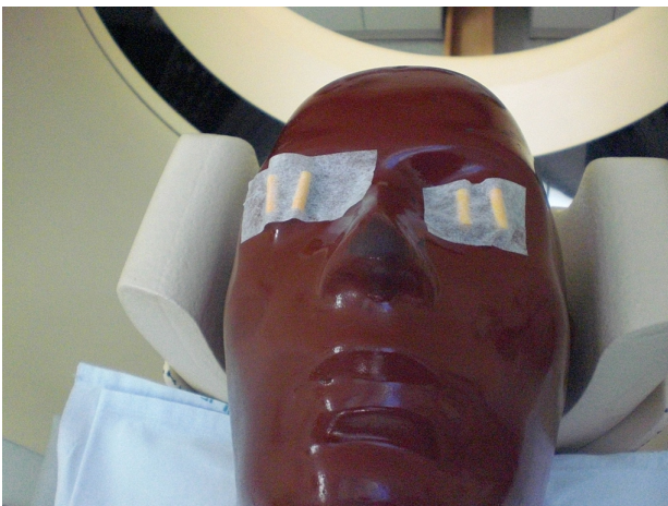
Figure 1. Photograph of anthropomorphic phantom with bismuth eye shield and glass dosimeters deployed
