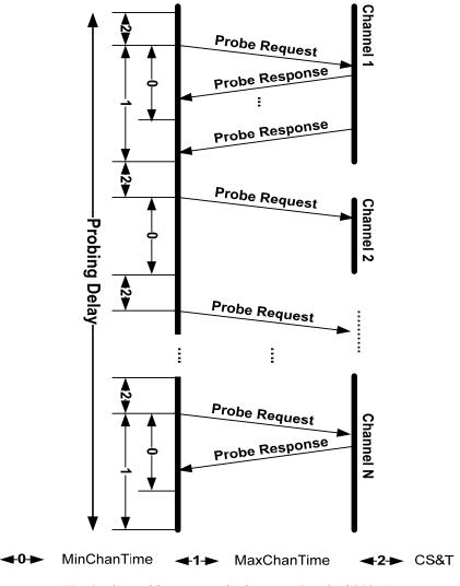
Fig. 4. The probing process in the IEEE Standard 802.11.
