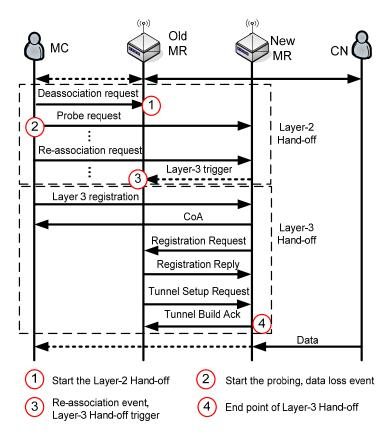
Fig. 7. The hand-off process with different buffering data moments.
