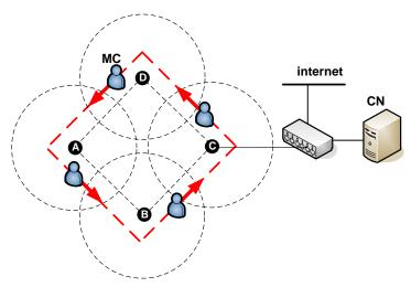
Fig. 10. The mesh network testbed topology.
