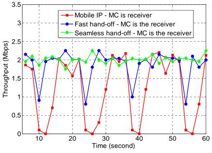
Fig. 13. TCP throughput observed at the CN node.
