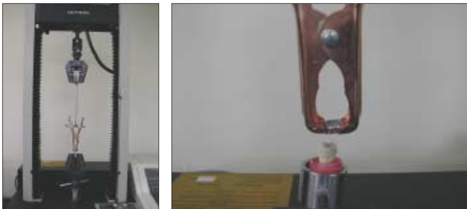
Fig. 1. Mounted tooth clamped to a customized holding device fixed to the load cell of the Instron machine.
