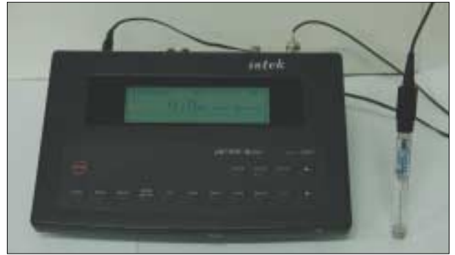
Fig. 4. Fluoride sensitive electrode and pH/ISE meter(Istek, Korea).
