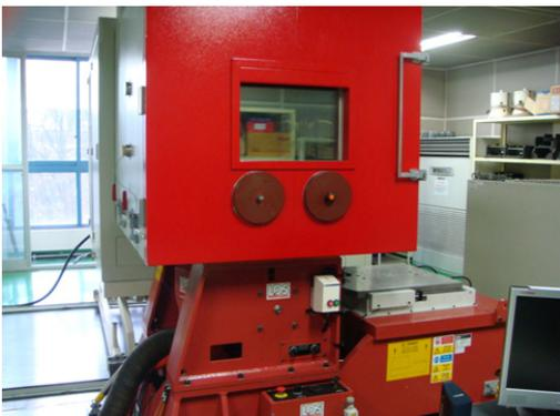
Fig. 4 Experimental setup for transmissibility test
