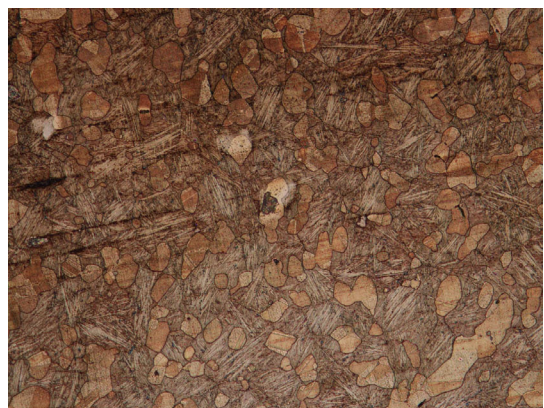
Figure 3. Microstructure of bronze spoon (Ga-5 tomb, x200).
