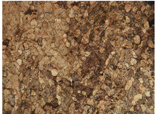
Figure 5. Microstructure of bronze spoon (Na-6 tomb, ×200).
