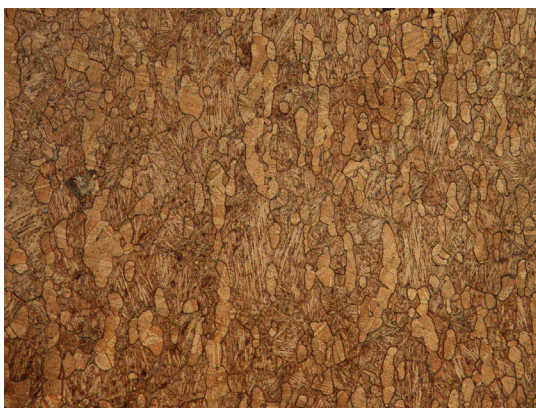
Figure 2. Microstructure of bronze spoon (Ga-2 tomb, x200).
