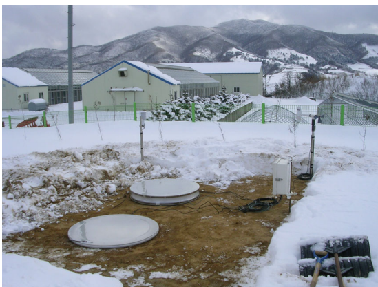
Fig. 2. Photograph of field installation of Rounded Snow Plate.
