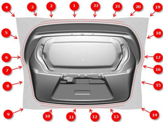
Fig. 8 Positions in liftgate draw panel for measuring draw-in amounts
