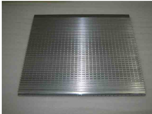
Fig 9. The fabricated configuration of this planar array antenna.
