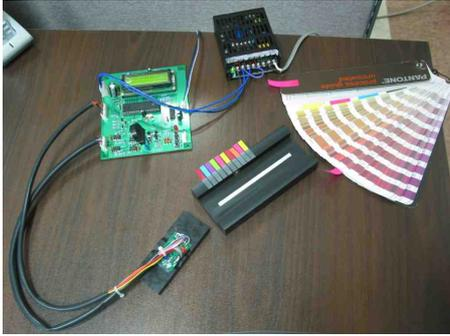
Fig 1. Hardware of primary color reaction for urine analyzer.
