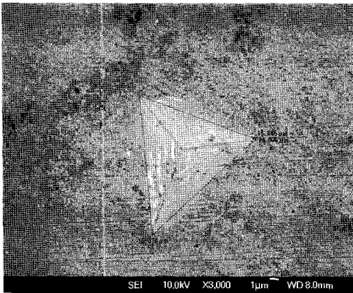
Fig. 7. SEM image of a indent for pure Ni at P=200 mN.
