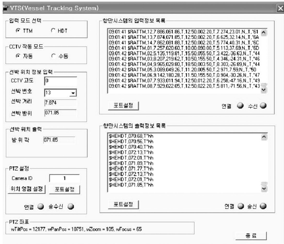
Fig. 4. A monitoring window of image tracker that is automatically being tracked the selected target vessel(No. 13) in response to the TTM signal(SRATTM) of vessel information receiving from ARPA radar. The bearing signal(SHEHDT) of vessel being tracked continuously by CCTV camera system is simultaneously being transmitted to the ECDIS in real-time.
