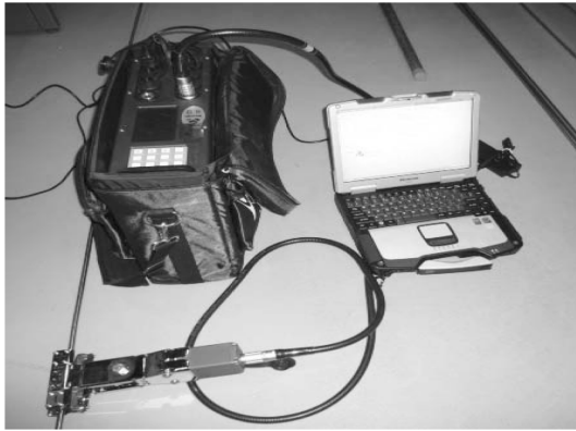
Fig. 4 Guided Wave Inspection System
