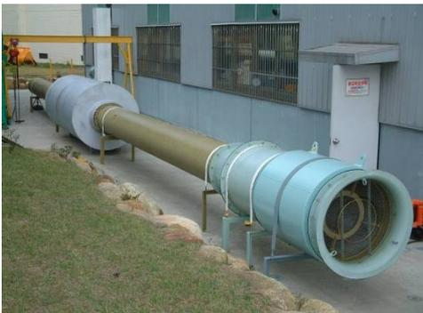
Fig. 2 Exhaust silencer test facility
