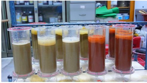
Fig 2. Columns filled with mixtures of tailings and inorganic binders
