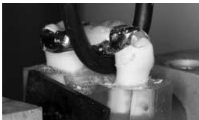
Fig. 6. The Specimen of group III, showing failure at the second premolar.
