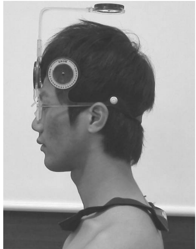
Figure 2. The CROM device has a transverse plane inclinometer to measure rotation, sagittal plane inclinometer to measure flexion/extension, and a frontal plane inclinometer to measure lateral flexion.
